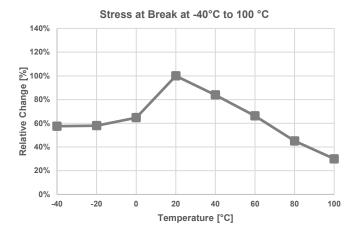
ASTM D638, Type IV, Pull speed: 5 mm/min, Young's modulus measured at 0.1-1% (regression)
