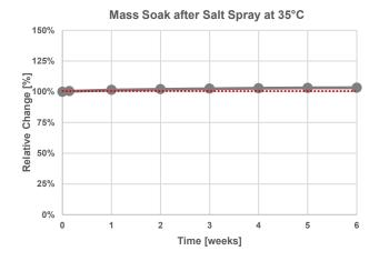
**Test parameters:** ASTM B117-19: pH = 6.1; Fog collection = 1.3 ml/h
