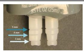
Turn syringe tips end up and pull plunger back slightly allowing air bubbles to rise to the top. Press the plunger to expel air. Depress the double piston to dispense equal parts of the two materials on a clean, discardable surface. Mix resin and hardener thoroughly for 1 minute. Wipe syringe tips clean, retract piston slightly and close syringe tips with plug provided to prevent leakage. Ensure that the plug is always placed in the same orientation on the tip.
