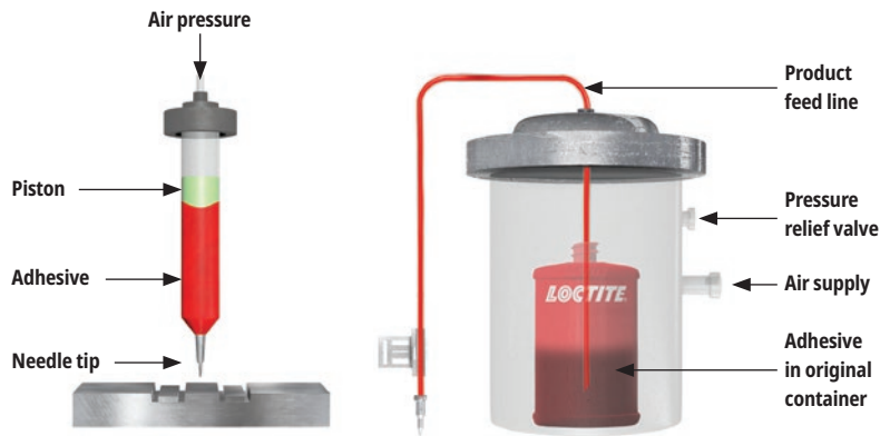
FIGURE 72 Pressure/time dispensing system diagram.
