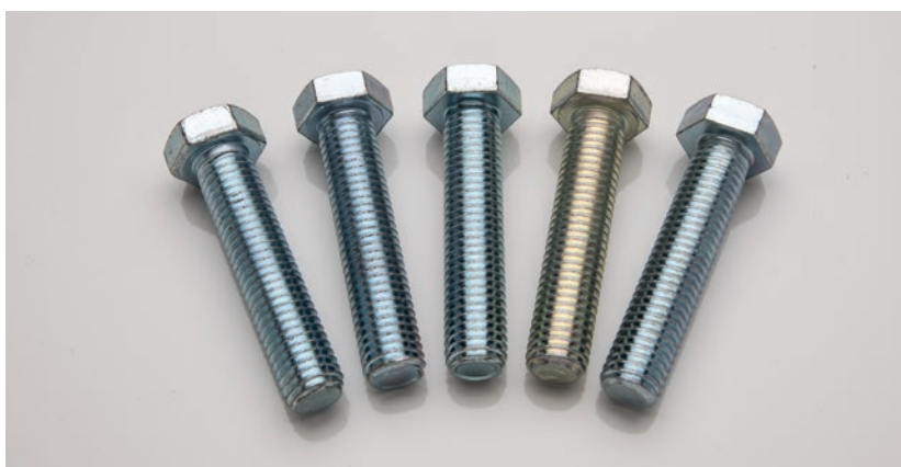
FIGURE 24 Visible variation in fasteners with the same specification from different manufacturers.
