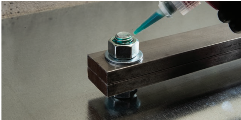
FIGURE 59 Proper post assembly application; wicking threadlocker.
