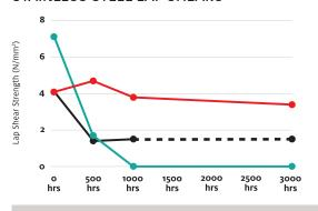
LOCTITE 402 VERSUS TYPICAL INSTANT ADHESIVES: HEAT AGED AT 135 °C AND TESTED AT ROOM TEMPERATURE ON STAINLESS STEEL LAP SHEARS
