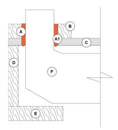
A and A1: Pro Gaps & Cracks Foam applied between gap at horizontal bottom wall plate framing and vertical penetration material. Gap between framing and penetration material must be a minimum of a ¼". Pro Gaps & Cracks Foam must fill gap. Do not cut expanded foam after cure.
