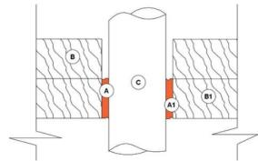
A and A1: Pro Gaps & Cracks Foam applied between gap at horizontal double top plate framing and vertical pipe. Gap between framing and penetration material must be a minimum of ¼" (6 mm). Pro Gaps & Cracks Foam must fill gap. Do not cut expanded foam after cure.
