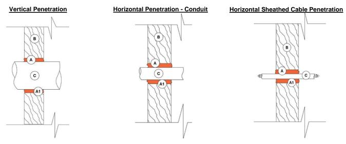
A and A1: Pro Gaps & Cracks Foam applied between gap at vertical framing and horizontal penetration material. Gap between framing and penetration material must be a minimum of ½". Pro Gaps & Cracks Foam must fill gap. Do not cut expanded foam after cure.
