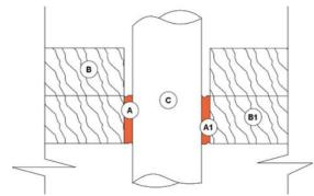
**A and A1:** Fire Block Foam applied between gap at horizontal double top plate framing and vertical pipe. Gap between framing and penetration material must be a minimum of ½" (6 mm). Fire Block Foam must fill gap. Do not cut expanded foam after cure.
