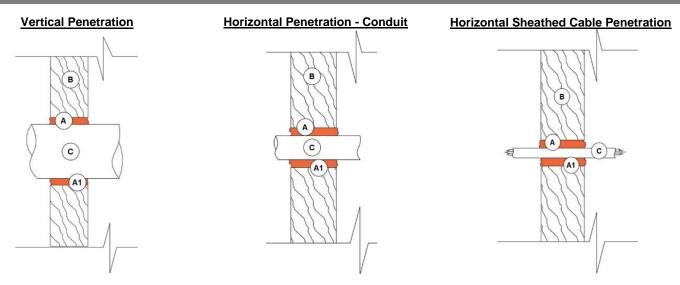
A and A1: Fire Block Foam applied between gap at vertical framing and horizontal penetration material. Gap between framing and penetration material must be a minimum of ½". Fire Block Foam must fill gap. Do not cut expanded foam after cure.
