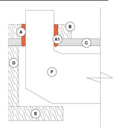
**A and A1:** Fire Block Foam applied between gap at horizontal bottom wall plate framing and vertical penetration material. Gap between framing and penetration material must be a minimum of a ¼". Fire Block Foam must fill gap. Do not cut expanded foam after cure.
