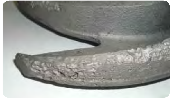
Worn impeller prior to repair.
