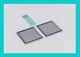
(H=50:50) and one low force sensitive zone (L=80:20). Printed designs determine system sensitivity due to the physically thin sensor format.
