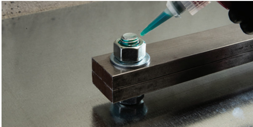
FIGURE 59 Proper post assembly application; wicking threadlocker.
