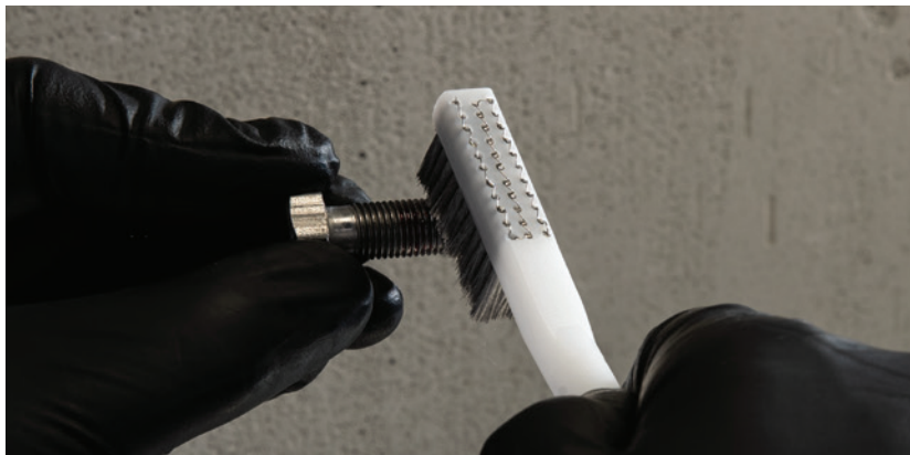
FIGURE 57 Cleaning a bolt with a brush.
