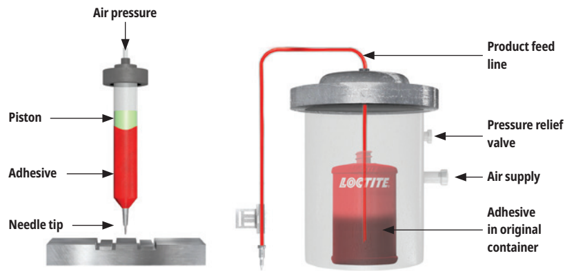
FIGURE 72 Pressure/time dispensing system diagram.
