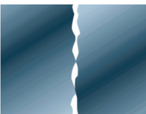
Typical interference fit has 30% metal-to-metal contact.
