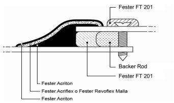
•Gutter joints and down spouts can be sealed with the Fester® FT 201 sealant or with Fester Vaportite® 550 in conjunction with Fester® Acriflex or Fester® Revoflex reinforcement meshes. The system must be complemented by Fester Vapotite® 550 and Fester® Festalum®.
