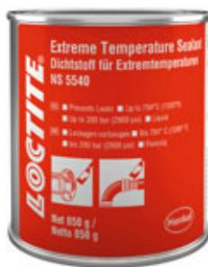
**LOCTITE NS 5540** is suitable for high pressure steam applications, this brushable liquid can seal flanges carrying up to 200 bar (2900 psi) steam at temperatures up to 700°C.
