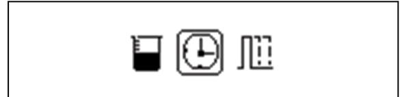
External time control operating mode is selected. ("Start/stop" or "continuous operation")
