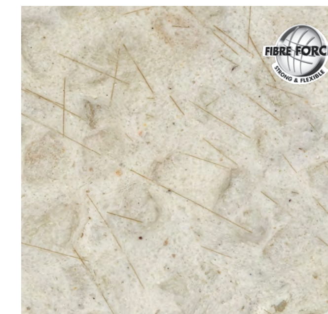
Microscope visualization of fibres inside the render
