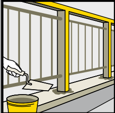
Assembly of fence elements
