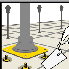
Fixing outdoor lampstand and street piles (columns)
