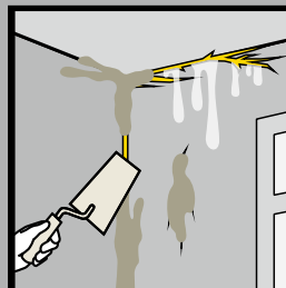
Crack repair and water leak protection – indoor
