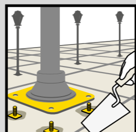
Fixing outdoor lampstands and street piles
