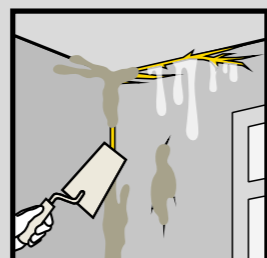
Crack repair and water leak protection - indoor
