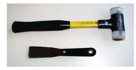
Dirt or fluids must be removed from the sealing surfaces. The product must be applied to a dry flange.
