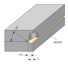
For this design, only the chamfer area has to be completely filled with RTV Elastomers.
