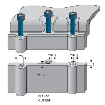
In addition to the correct design of the flange, reliable sealing with FIP gaskets depends on adhesion to the flange surface. The adhesion is strongly influenced by the cure performance. The anaerobic cure starts when atmospheric oxygen is excluded. Then free radicals are formed and under the effect of metal ions (Cu, Fe), these free radicals initiate the polymerization process.
