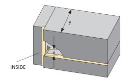
The dimension x always has to be smaller than the overall flange width y. Common dimension: x = 3 mm (y-x > 3 !) The minimum recommended flange width y is 10 mm.
