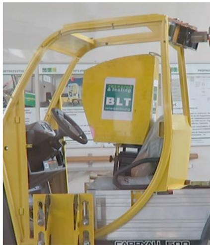
**Figure 5** > Load case 1 of ROPS test
