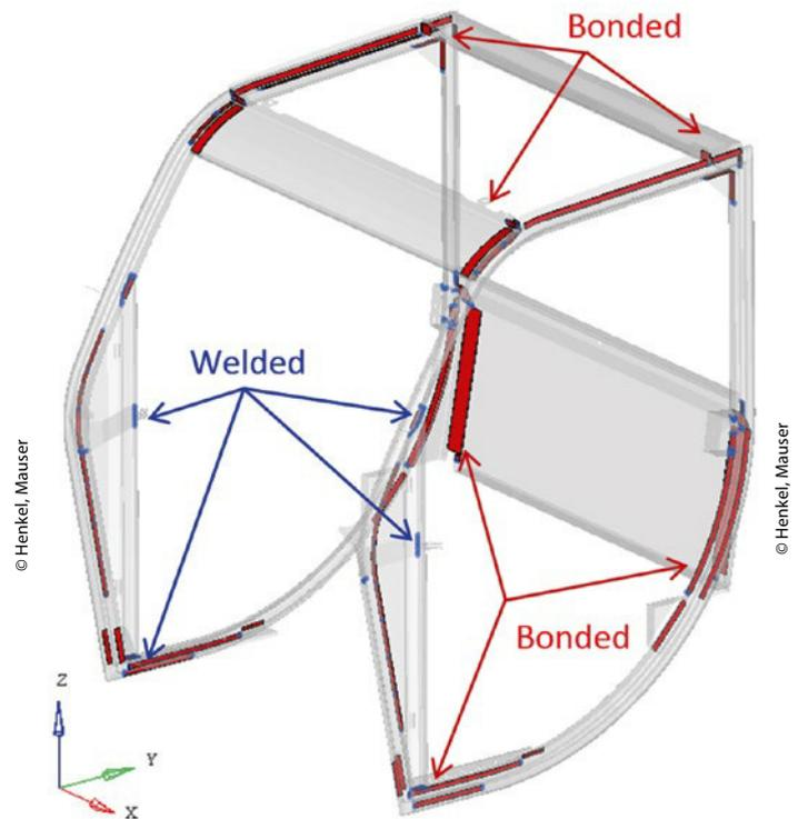
**Figure 2** > Redesigned areas of the CAD model
