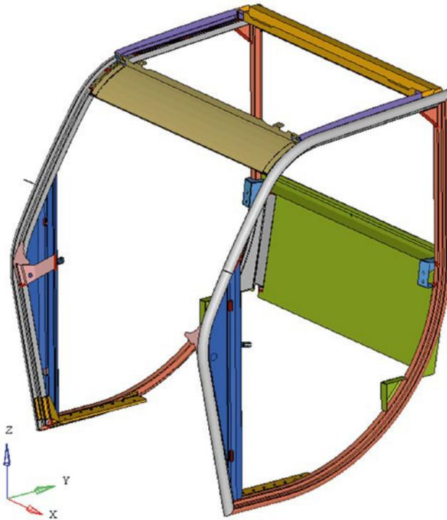
**Figure 1** > CAD model of the cabin frame
