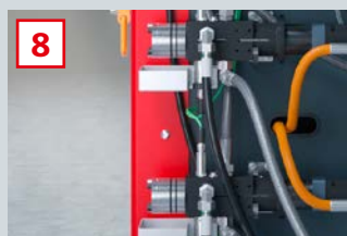
Precision gear pumps with 0.75 ccm/rev delivery rate of the A and B components of the 2K silicone systems
