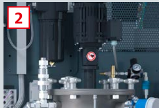
Agitator for homogenization of the A component
