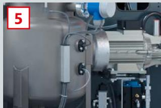
5 Capacitive sensors for filling level regulation
