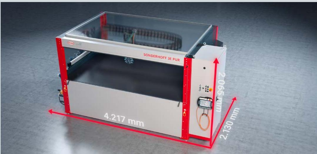
The dosing cell can be used flexibly as a production island, and with an installation footprint of approx. 9 square meters requires very little space.
