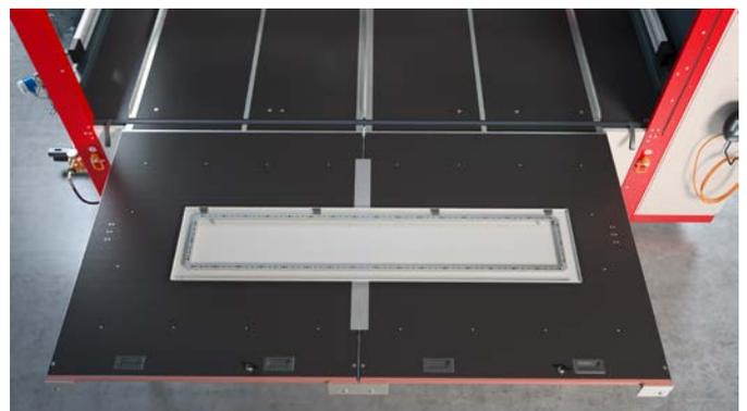
The two mounting plates are connected by couplers to form one large sliding table.
