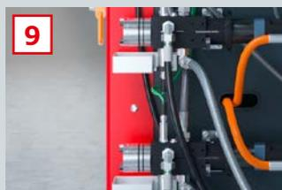
9 Precision gear pumps with flow rate 0.75 ccm/rev (material component A) and 0.3 ccm/rev (material component B)
