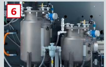
6 Material pressure tank with optimized dimensions for asymmetrical mixing ratios
