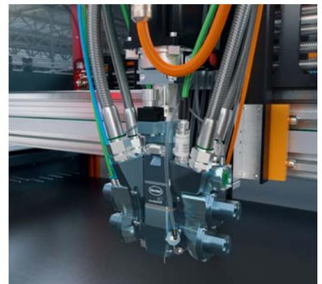
Standard equipment: MK 825 BASIC precision mixing head for 2 components, with high-pressure water rinsing
