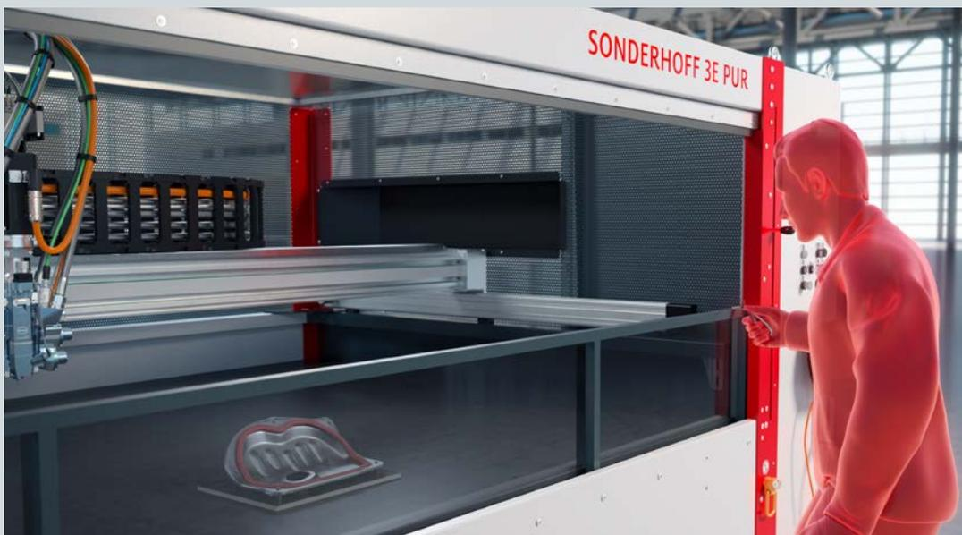
To remove one or more parts after the dispensing process, the machine operator opens the lifting door using either the hand strap mounted there or the lever.
