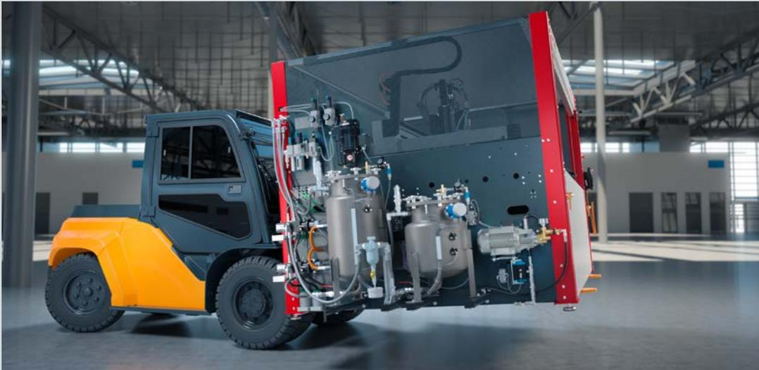
The dosing cell is removed from the transport container, set up and connected: place, plug & work. All features are arranged on a single chassis so that the dosing cell can be changed over very easily in production.
