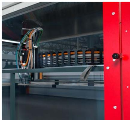
Half-open lifting door shows MK 825 BASIC precision mixing head and energy chain
