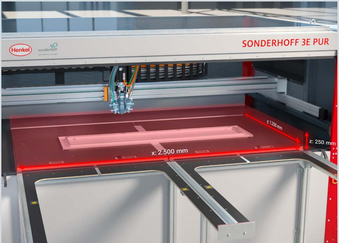
In order to be able to produce oversized components with a maximum dimension of 2,500 x 1,250 x 250 mm (x/y/z), the two sliding table plates are joined together to form one large mounting plate.
