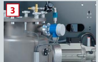
3 Overfilling protection for the use of an optional refilling station
