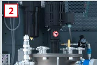
2 Agitator for homogenization of the material component A
