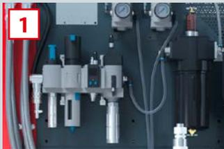
1 Compressed air connection, dryer and maintenance unit
