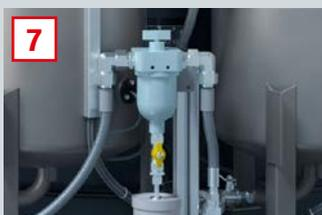
7 Plate gap filter for the material component B
