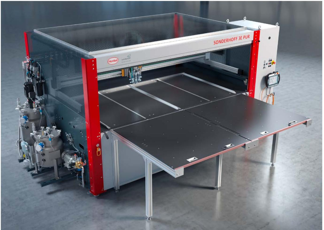
The SONDERHOFF 3E PUR dosing cell offers an attachable sliding table with manually shifting mounting plates as an alternative option for placement and processing of industrial parts for sealing, bonding, or potting. With this solution, a machine operator loads the two mounting plates with the parts in an alternating sequence. The parts are positioned in workpiece fixtures, which are fastened on the mounting plates made of coated multiplex.
