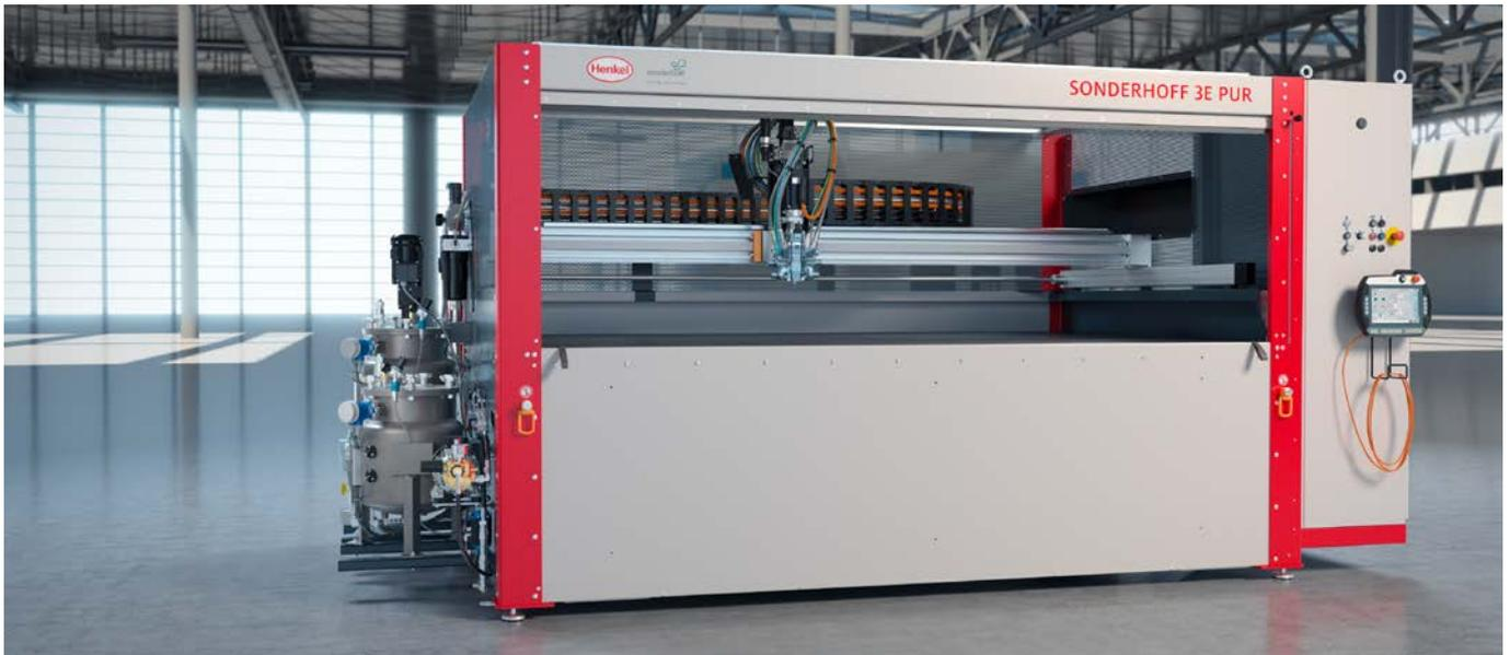
The SONDERHOFF 3E PUR dosing cell comprises the MK 825 BASIC precision mixing head for 2-component products with high-pressure water rinsing for mixing chamber cleaning. In the mixing head the material components are mixed dynamically, and the material system to be applied to the part is dosed in precise quantities. The MK 825 BASIC enables dosing from 0,2 to 3,0 g/s with continuously adjustable, asymmetrical mixing ratios from 10 : 1 to 1 : 2 and a dosing accuracy of  $\pm 1\%$ .
