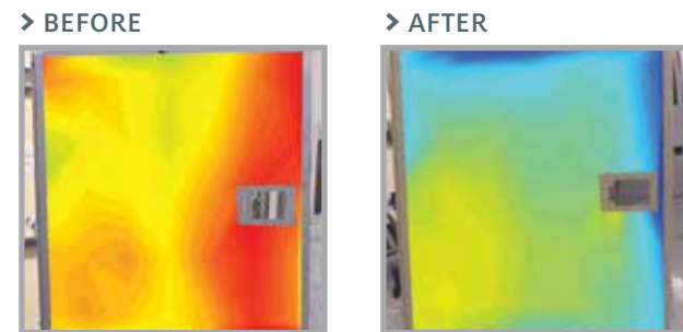
Vibration response test for side panel. Red/yellow indicates high levels of vibration.
