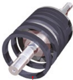
Ring magnets to rotor
