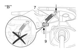
Assemble Spring 7 correctly, to prevent its jumping out, when the Adjusting Screw 9 is turned
