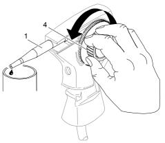
• Priming the Pump: Turn Dispense Wheel **4** CCW, until the product comes out of the Nozzle **1**
