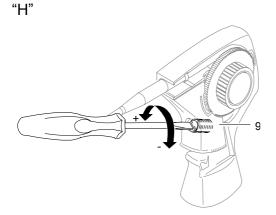
The dispense amount depends on the stroke adjustment of the Trigger **8**.
