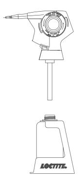
4. Screw hand pump onto the bottle until it fits tight to the bottle (ca. 1.5 Nm). At the right positioning of the thread start, the hand pump is orientated as shown below. If the hand pump shows vice versa, unscrew the hand pump, turn the bottle 180° and screw the hand pump on again.
