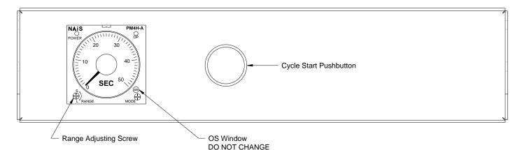
5. Turn on the power switch, and test that the shutter is cycling to the new time.
