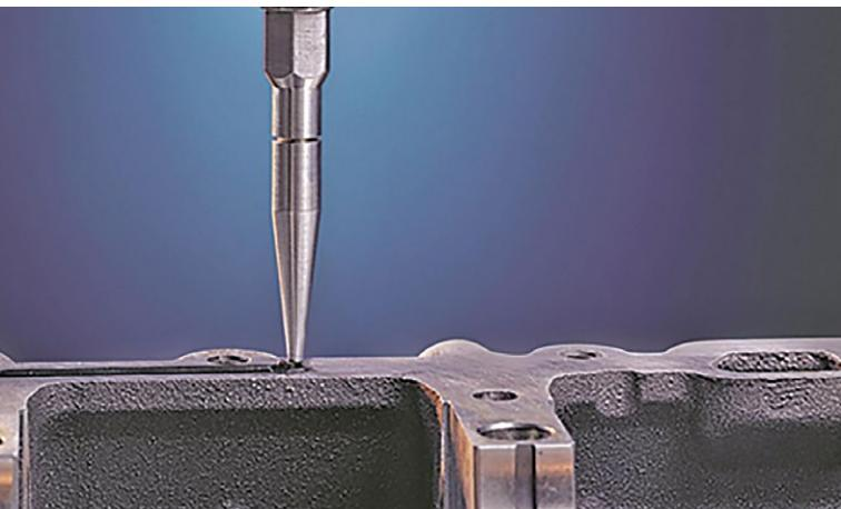
Form-in-place gasketing materials can eliminate the need to keep cut or molded gaskets in inventory. Better still, the process of applying the material can be automated.
