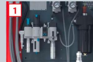
Compressed air connection, dryer and maintenance unit
