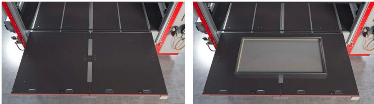
The two mounting plates are connected by couplers so that one large sliding table can be formed.
