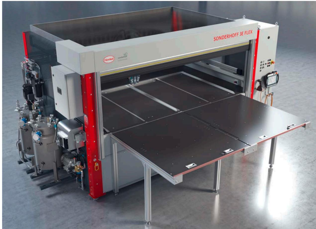
The parts can also optionally be loaded via an attachable sliding/shuttle table by manually moving the mounting plates.
