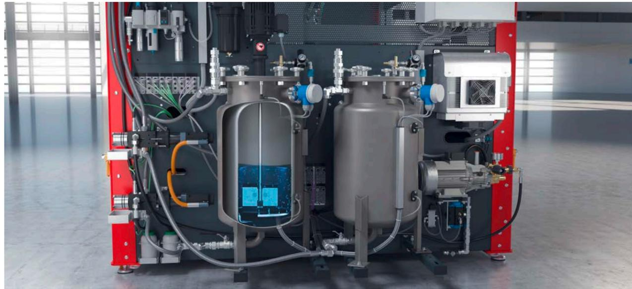
The **air loading** in the material pressure tank helps to create the desired physical properties and cell structure of the foam. The density can be influenced by adding compressed air to the material component.
