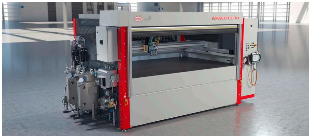
The MK 800/825 PLUS precision mixing head is used in the SONDERHOFF 3E FLEX dosing cell for processing a 2K material system. In the mixing head, the material components are mixed dynamically and homogeneously and then precisely dosed for application on the component. The MK 800 PLUS has a dosing capacity of 3.0 to 100 g/s and the MK 825 PLUS from 0.2 to 3.0 g/s, with an infinitely adjustable mixing ratio of 10 : 1 to 1 : 2 and a dosing accuracy of  $\pm 1\%$ .
