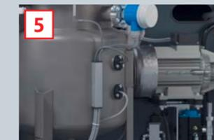
Capacitive sensors for filling level regulation
