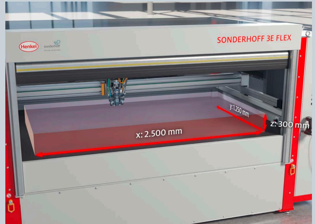
To produce oversized parts with a maximum dimension of 2,500 x 1,250 x 300 mm (3E FLEX) the two sliding table plates are joined for one large mounting plate.
