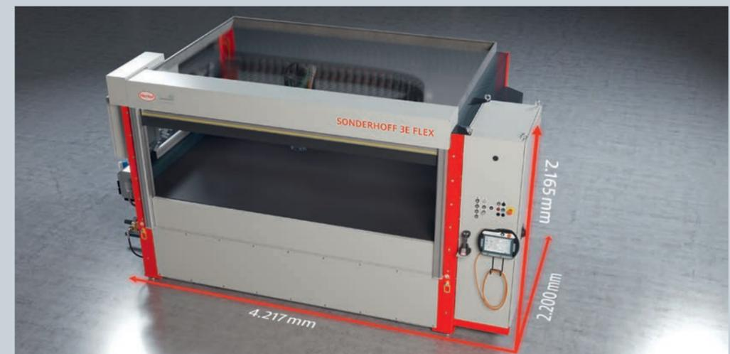
The dosing cell can be used flexibly as a production island with an installation footprint of approx. 9 square meters.
