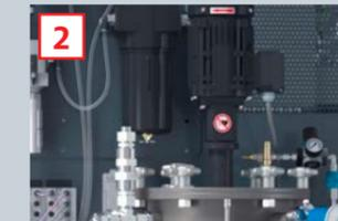
Agitator for homogenization of the A component
