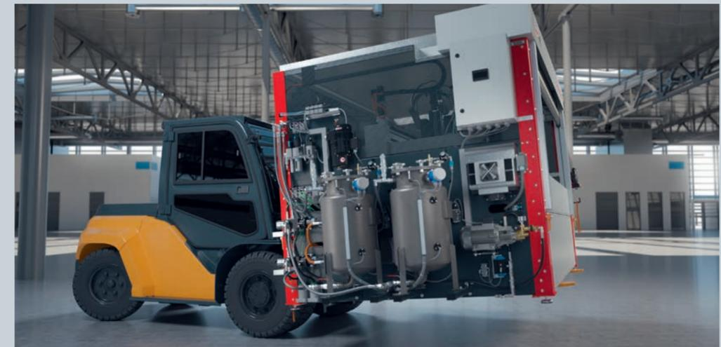
The dosing cell is removed from the transport container, set up, and connected: place, plug & work. All features are arranged on a single chassis so that the dosing cell can be changed over very easily in production.
