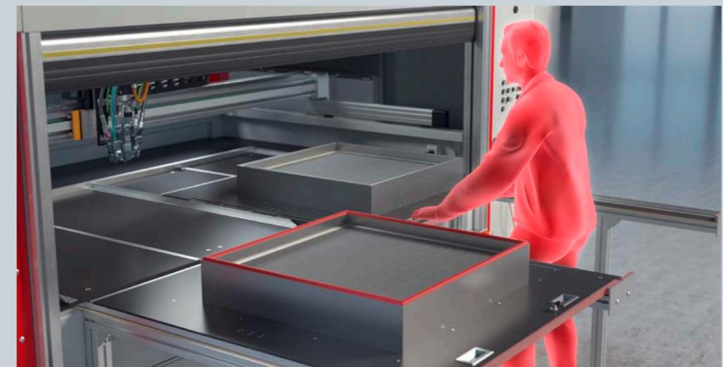
After the dosed application, the machine operator opens the high-speed door and pulls the sliding table with the finished parts out of the working area for removal.
