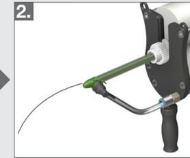
2. Increase fluid flow until you are able to achieve a good fluid stream. Ideally 50-75mm (2-3 in) before arcing downward.
