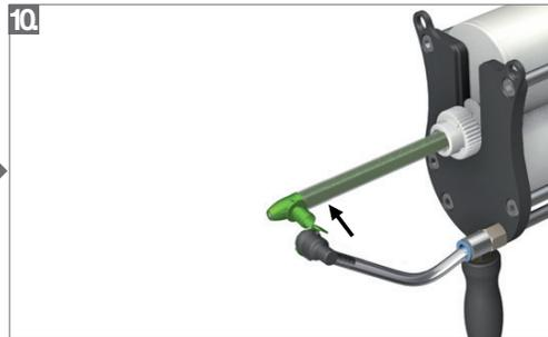
10. Connect atomizing air line to spray nozzle.
