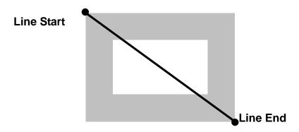
If, for example, a brush width of 5 mm and band of 10mm was used, the tip will take the following path when the program is run:
