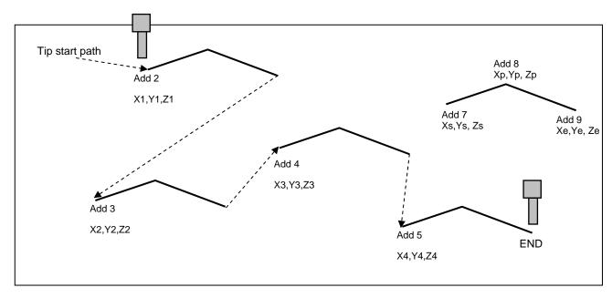
Addresses 7, 8 and 9 comprise the subroutine that will be executed whenever it is called within the main program. The coordinates in the body of the subroutine (Xs,Ys,Zs, Xp,Yp,Zp Xe,Ye,Ze) are not important; *the critical information is the relative position to each other*. The actual work will be performed on the coordinates in the main body of the program.
