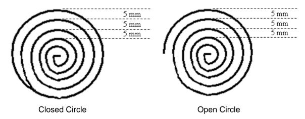
An open or closed option is also available for this function. Selecting the Closed option will make a whole circle first before making the spiral. Selecting the Open option will make the spiral without closing the outer circle.
