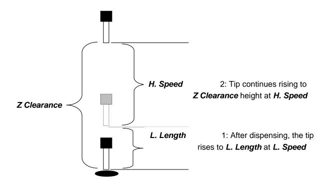
Values for *H. Speed*, *L. Speed* and *L. Length* are registered with the *Dispense End Setup* function by pressing the **F4** key, then choosing **Dispense End Setup**.
