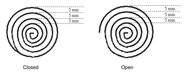
An open or closed option is also available for this function. Selecting the Closed option will make a whole circle first before making the spiral. Selecting the Open option will make the spiral without closing the outer circle.
