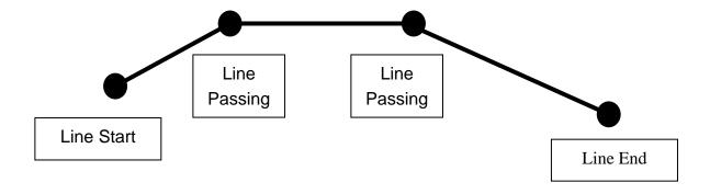
To dispense a bead of material in an arc, the XYZ location of the start of the line is registered as a LINE START point type. The high point of the arc is registered as an ARC POINT. The end of the arc is registered as a LINE END point:
