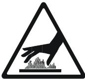
**WARNING:** During operation the lamp bulb and adjacent metal surfaces become very hot. Operate the blower for about one minute to cool hot surfaces.
