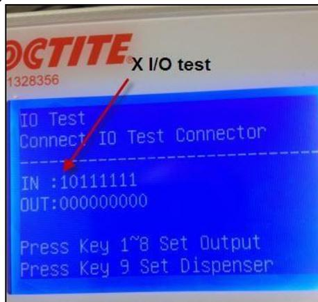
**Figure 8:** X I/O test.
