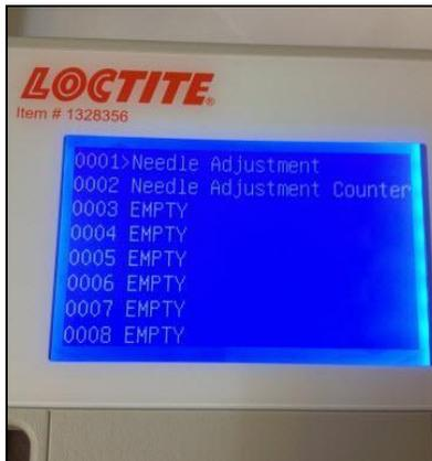
**Figure 7:** This is how the memory address screen will look after programming the Needle Calibration Kit is complete. **\*\*\*Note Address 1 and 2 are reversed in this picture\*\*\***
