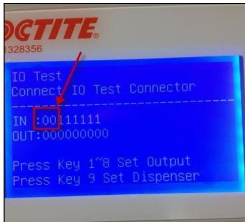
3) Take a dispense needle in your hand. Manually put the needle down in the calibrator and move back and forth in front of the X sensor (right and left). You should see a 1 appear in the first digit when the needle crosses the sensor. See **Figure 8** below. Repeat for the Y & Z sensor (forward and backwards), you should see a 1 in the second digit.
