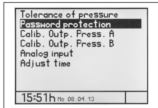
“On” is automatically marked. It means, the password protection is switched off (“Protection inactive”, see status bar) and by pressing button **8** *ENTER* it is switched on and vice versa.
