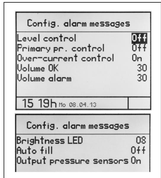
If the level sensing function is activated as ON, (happens automatically when connecting a product reservoir) and the reservoir fill level drops to the low-level set point triggering a low level signal, the controller will not permit the Dispenser to start another dispense cycle.
