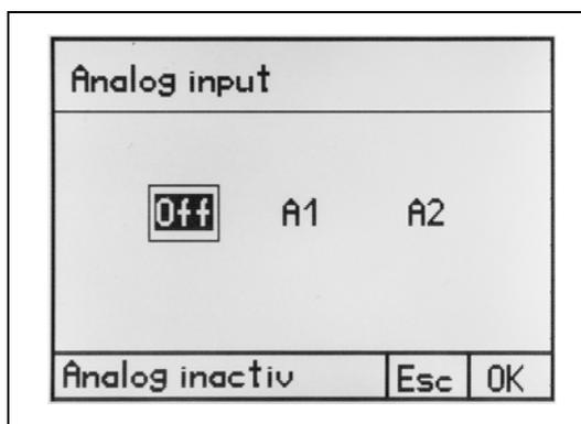
A1: 0-10 V DC, corresponds to 0-6 ml/min max. flow rate (A+B, independent of the ratio)
