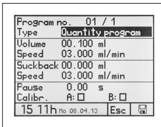
To select and adjust each setting use selector **2**, button **8** *ENTER* and button **6** *PRG/ESC*, see section 2.5.
