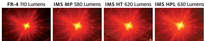
Light output of the same LED die on different circuit board materials at a maintained die temperature of 80°C.
