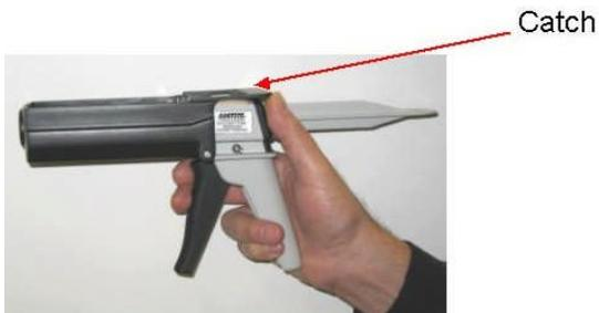
**Step 2.** Drop in the adhesive package. Return the tray to original position and snap catch back into place.
