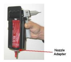
Note: When dispensing PST products from a ribbon tipped package, remove nozzle adapter and place it into the nozzle adapter holder located on the underside of tray.
