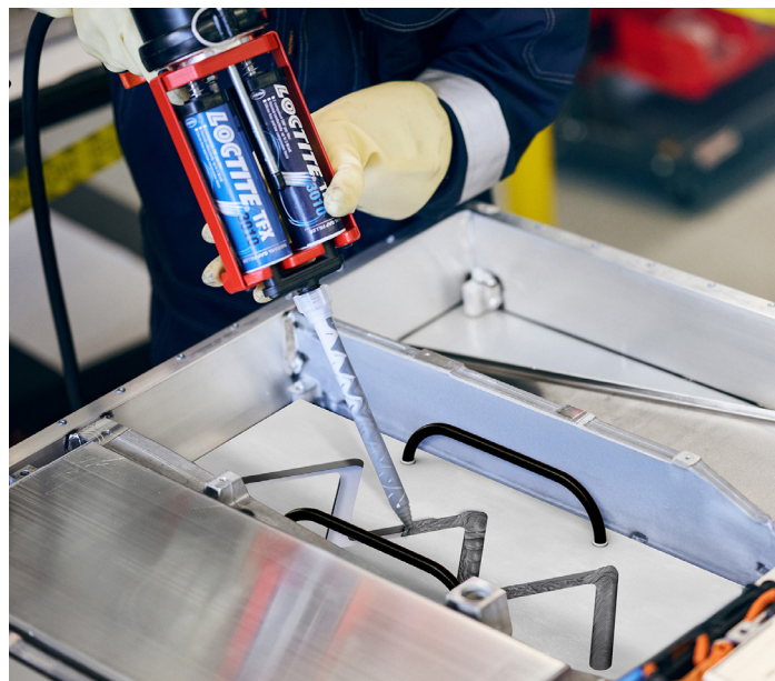
LOCTITE TFX 3010 THERMAL GAP FILLER APPLICATION
