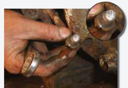
...which can lead to broken bolts.
