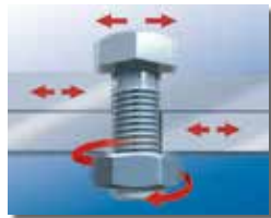
Vibration and loosening.
