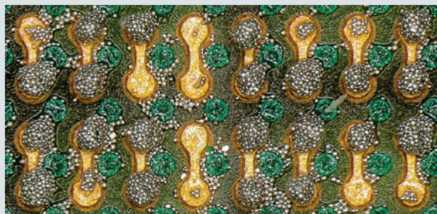
0.3 mm CSP printing: Competitive paste's poor transfer efficiency results in high solder volume variability and the potential for defects.
