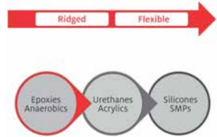
Figure 3: Generalization of flexibility expected from various adhesive product chemistries.
