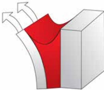
Figure 2: Example of Peel Force
