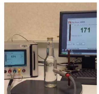
Our Oxygen Scavenging Technology (OST) provides a solution to problems of oxygen ingress during the filling process and oxygen ingress over time. This technology can be used in several applications, including lined crowns for beer bottles, aluminum RO/ROPP or in the center panel within plastic caps. In addition, an OST masterbatch has been developed to be incorporated in other packaging type.
